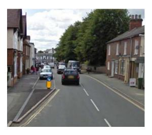
Single lane chicanes require one direction of traffic to give way to oncoming vehicles. The chicane normally consists of a raised kerb and bollard in one half of the road, with a sign to explain the vehicle traffic priority. For the lane without traffic priority, there are Give Way markings and hatching on approach to the chicane. They are most effective if used by more than 500 vehicles a day, with no heavy bias in one direction.
